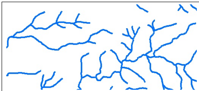
Fig. 2.5 Parallel drainage pattern in Palar sub basin
